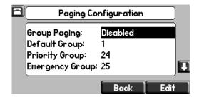
1 Make your changes to the paging configuration by highlighting a setting and pressing the **Edit** soft key.
